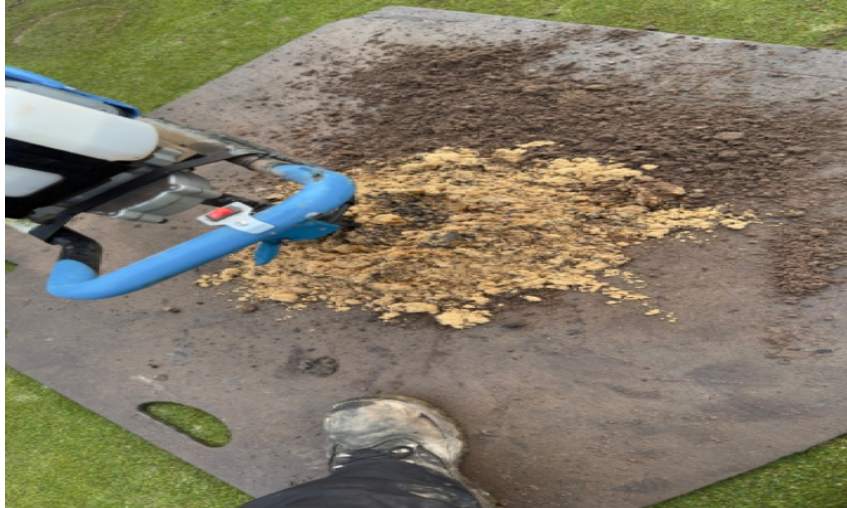
Figure 1: Brown material on the board is clay, the yellow is sand
